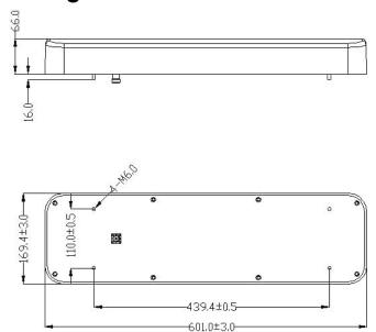
BRA-21 can be used outdoors, but it is not suitable for use in acid/alkali environments. The bracket is an optional accessory.
